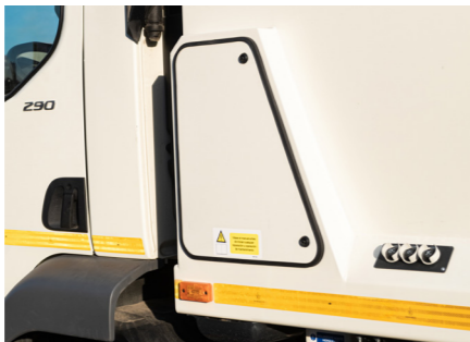
5 Easy access electrical control panel
