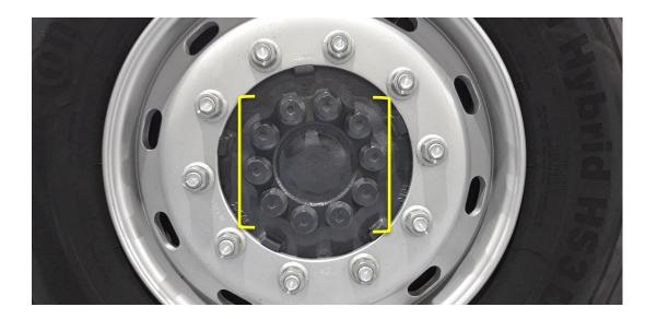
Dennis Eagle recommend that on the vehicles next planned inspection, the hub bolts are physically torqued to the new value of 500Nm and the bolt security is then checked and maintained on the vehicles six weekly safety checks.
