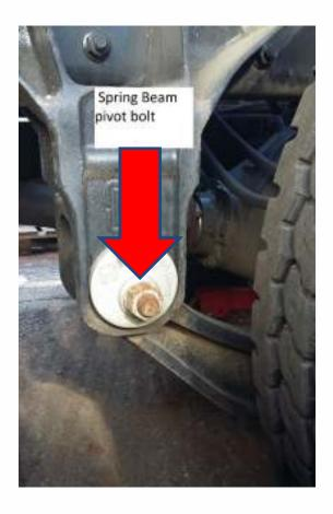
The bolt pointed out in Fig.1 should be torqued 540-660Nm (398-486 lbf-ft).
