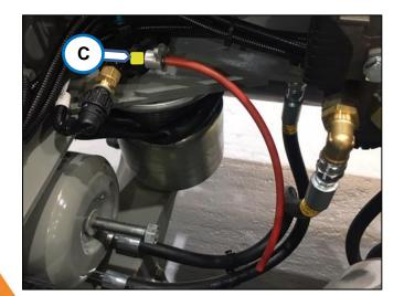
C. Open ended pipe screwed onto an air bag pressure test point.
