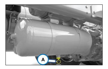
A. Manual air tank drain valve, pull to drain air from each tank.
