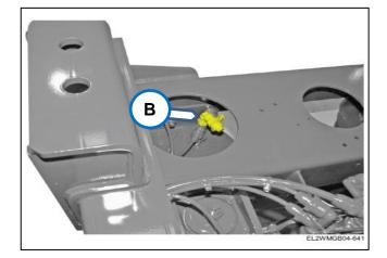
B. Example of air bag pressure test point.
