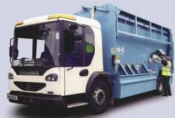
The Terberg kerbsider mounted on the Elite 4 x 2 chassis
